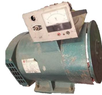
Gambar 2.3 Generator Sinkron
