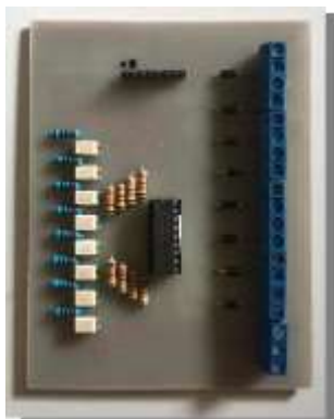
Gambar 7 Desain Driver Relay ULN 20803
